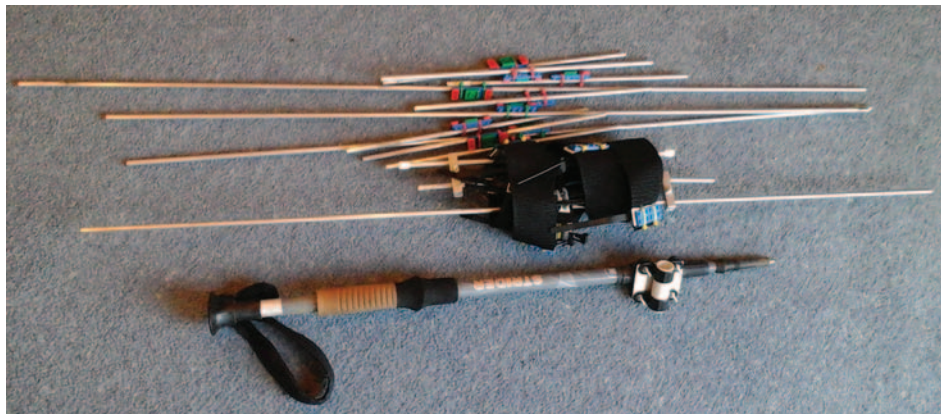
PHOTO 2: Earlier roll-up dual band Yagi, ready for transport. The walking pole in the foreground shows the mounting bracket.
