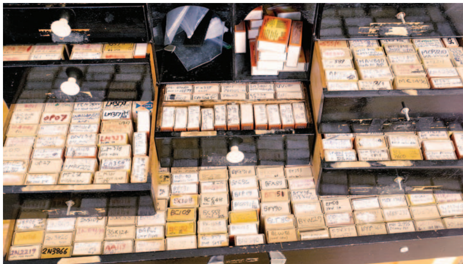
PHOTO 1: Part of the 'JNT semiconductor junk box that started in 1973. Devices are stored in individual labelled matchboxes, some of which may be more valuable as antiques than their contents.
