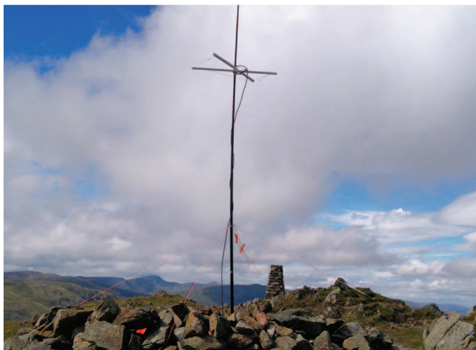
PHOTO 4: Lightweight Moxon mounted on our guyed fiberglass fishing rod atop Red Screes.
