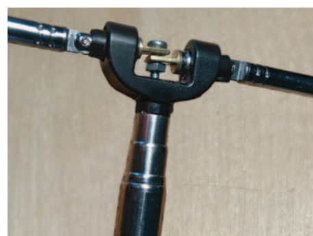
PHOTO 5: C-shaped bracket adapted to mount the reflector.
