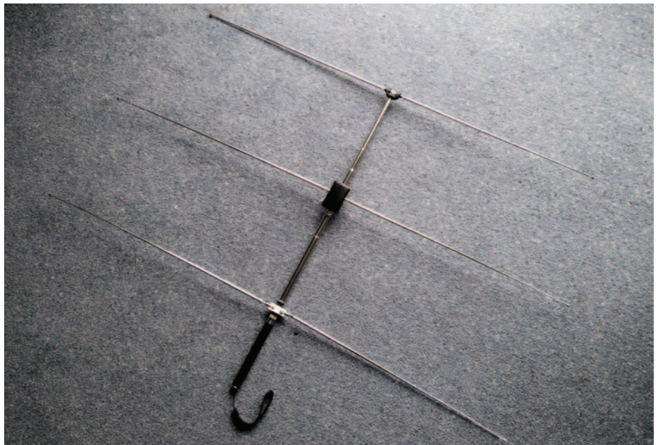
PHOTO 1: The prototype selfie-stick antenna.
