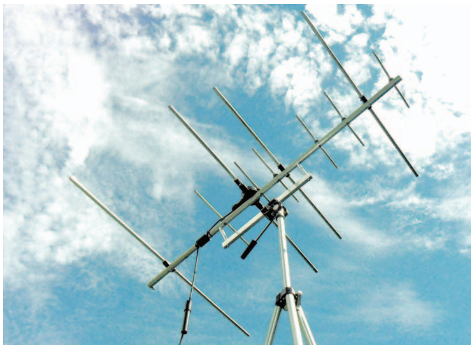
PHOTO 1: The 2m/70cm dual-band beam in use. The tube in the coax contains a BNC joint.
